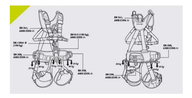
The VERTIC TRIPLE LOCK has four rigid gear loops for up to twelve carabiners each for transporting and organizing equipment, various attachment possibilities for equipment holders, first aid kit, work positioning seat and tool bag, as well as two loops on the chest harness for accommodating the carabiner for a lanyard. It is equipped with an integrated RFID chip, making deployment documentation easy to do and not just a necessary evil.
