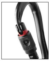
The integrated keylock closure prevents the carabiner's nose from catching on structures or the gear loop when being attached or detached. A red mark on the carabiner's gate furthermore indicates whether the carabiner is completely locked.
